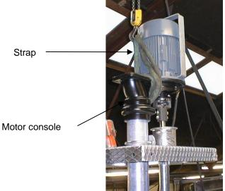
If the pump is to be hoisted horizontally, two straps/chains must be placed around the pump pipe.
