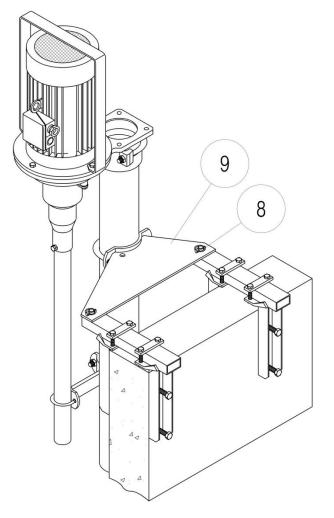
The pump is adjusted so that the guide pin is on the tank bottom, by loosening and tightening the nut, pos. 10.
