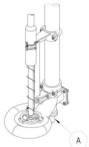
The checker plate cover with brackets must be adjusted on the pump pipe by loosening the nuts, pos. B, on the threaded shackle, pos. A.
